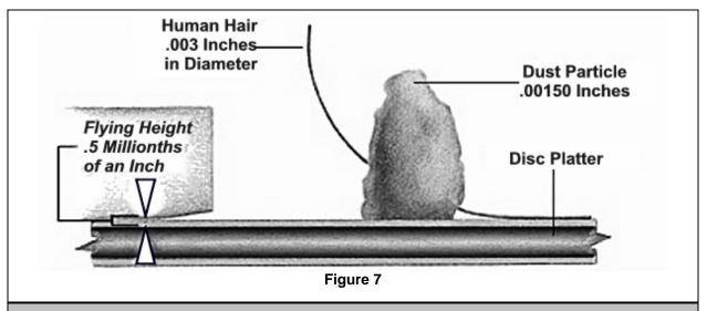
**Perspective:** Woody Monroy, head of corporate communications for hard drive maker Seagate Technology, L.L.C., points out that, in terms of speed and tolerances, a hard drive's operation is equivalent to an *F*-16 jet fighter plane flying at 813 times the speed of sound and one-sixty second of an inch off the ground...while counting every blade of grass as it goes!
