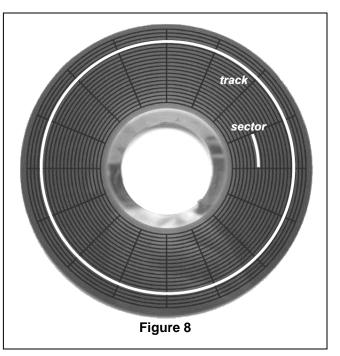
divided into tracks and sectors. In reality, the number of tracks and sectors is far, far greater. Additionally, the layout of sectors is no longer symmetrical, to allow the inclusion of more sectors per track as the tracks enlarge away from the spindle. Today's hard disks can have thousands of sectors in a single track and make use of a space allocation technique called zoned recording to allow more sectors on the larger outer tracks of the disk than on the smaller tracks nearer the spindle.
